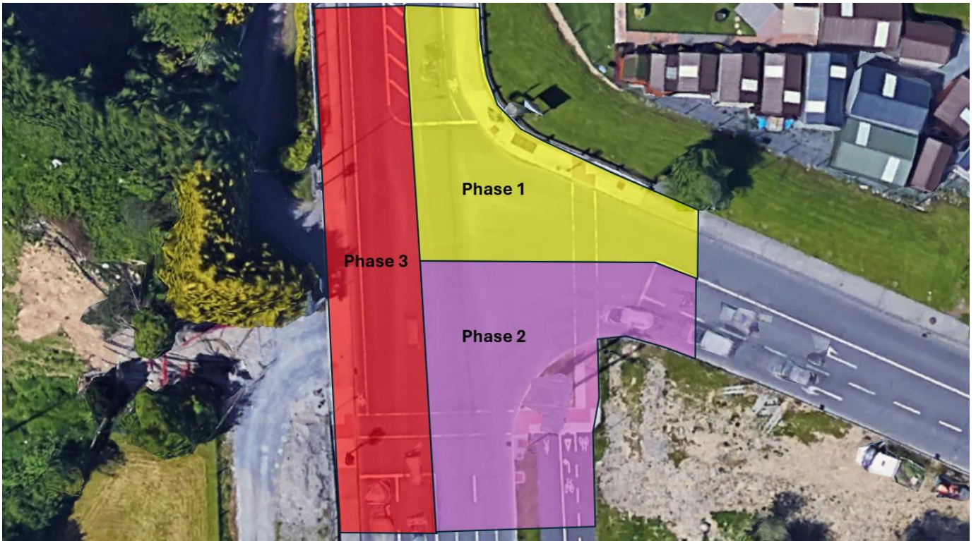
Figure 7-3 – Phasing of Works for Typical T-Junction
