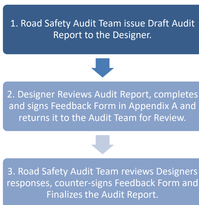
Figure 4.1 – Road Safety Audit Sign-Off and Completion Process
